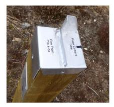
Using the bracket is very simple, just place you camera onto the bracket pointing in the direction of the view. This is marked on the bracket. Make sure the camera is carefully set against the back and left hand upright of the bracket and press the shutter button!
